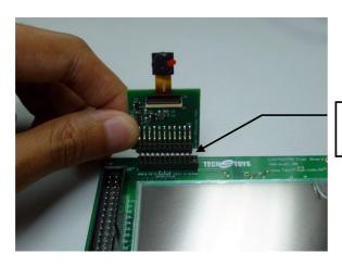
Install by swifting cmos camera module to the left
