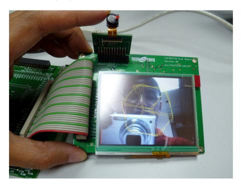
To display JPEG/BMP images from the microSD, press BUTTON0. The program will go back video display after cycling all images on the microSD.
