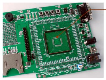
No mcu soldered here, leaving only 1.27mm 100-pin header for PIM
