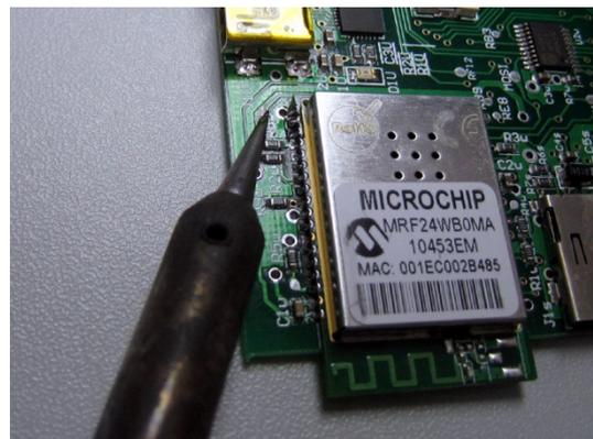
Figure 3-1. Solder MRF24WB0MA/B on MMEVK
