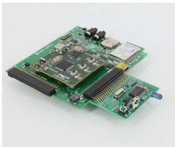
A PIC32 GP Starter Kit is stacked on board. Wireless LAN module MRF24WB0MA soldered, with an application module for universal learning IR plugged in the 2x22 2.00mm receptacle (JP2k). The 2.00mm receptacle has been designed to bring out most of the critical I/O pins of the PIC32 MCU including SPI, I2C, PMP, UART, and ADC, to name a few of those.
