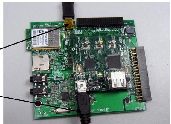
Figure 3-2. Hardware setup for wireless LAN demo
