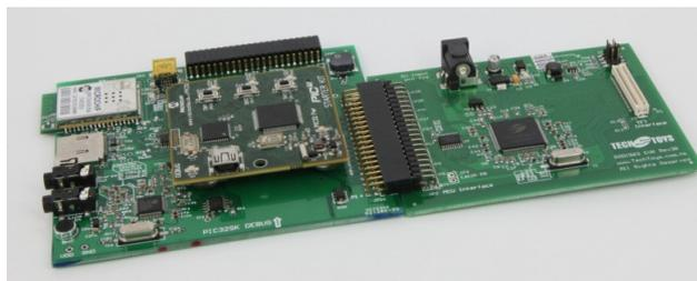
A PIC32 General purpose Starter Kit is stacked on board. This time, SSD1963 EVK is connected for applications requiring a graphical user interface up to 7" TFT with touch panel.
