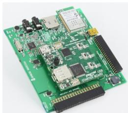
A PIC32 USB Starter Kit is stacked on MMEVK. The same socket can be used for PIC32 GP Starter Kit or PIC32 Ethernet Starter Kit. A wireless LAN module MRF24WB0MA has been soldered for internet applications.
