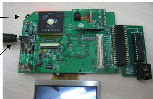
**Important:** Apply 5V @ 1A, better to use a regulated supply as it is a 6.3V tan cap (C507) in front of the 3.3V LDO (U502)
