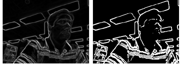
Fig. 5(a). Gradient Approximation of Image using Sobel kernel
