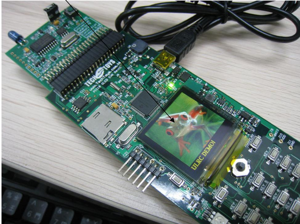
4. Important: use battery to power the board. This is because the ULRC device sources power from EXT VIN pin, which are connected to batteries of the OLED demo kit.
