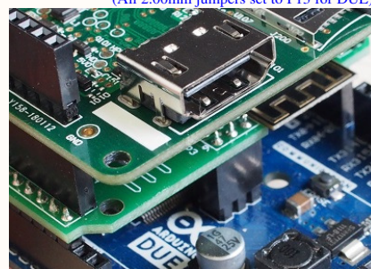
Direct stack HDMI shield to DueZipper for ESP8266 Soc (All 2.00mm jumpers set to P12 for ESP8266)
