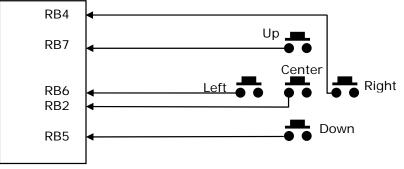
Remarks: keys' pins short to ground to read 0 when pressed
