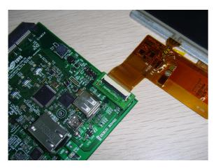
Resistive touch panel works like a potential divider. Measuring a touch position is actually to measure the voltage at XR and YU when a DC voltage applied in the direction YU(+ve)-YD(-ve) and XR(+ve)-XL(-ve), respectively.
