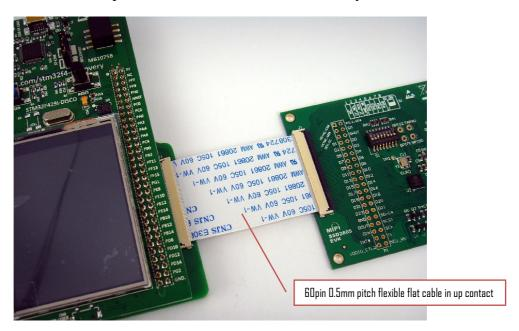
Wiring to the application module is finished with a 40pin 0.5mm pitch FFC.
