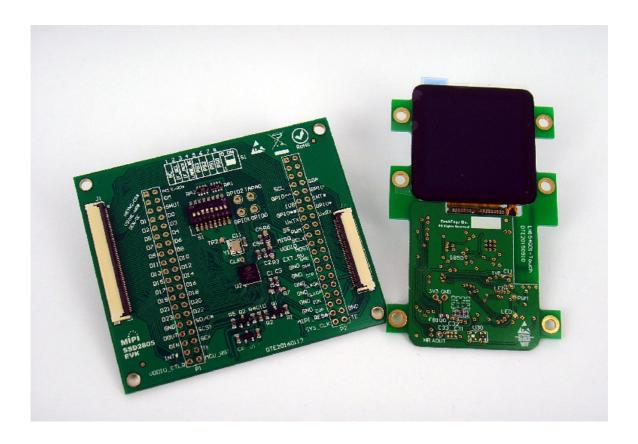
SSD2805 MIPI Master Bridge breakout board has been routed with simplicity in mind. Pixel data from an application processor (MCU/MPU) in RGB/8080 data bus is fed to the 60 pin FPC connector J1 from the left. After conversion and protocol translation finished by SSD2805, differential signals that conform to DSI specification is output through a 40 pin FPC connector J2 at the right.
