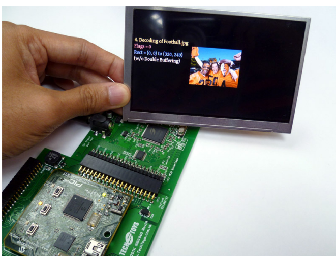
Figure 2 Development platform MMEVK R1A with Microchip PIC32GP SK on board
