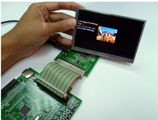
Figure 1 Development platform PIC23/32 EVK RD4 with PIC32MX360F512L MCU option
