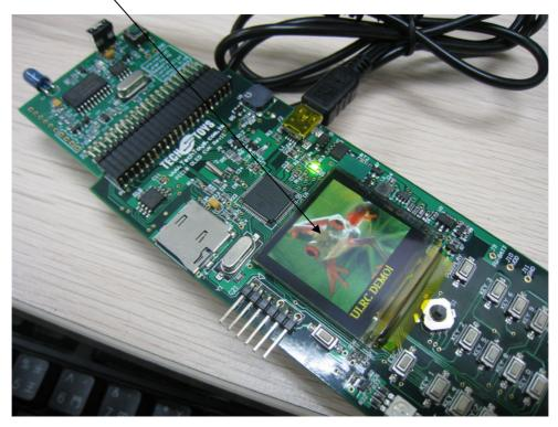
4. Important: use battery to power the board. This is because the ULRC device sources power from EXT VIN pin, which are connected to batteries of the OLED demo kit.
