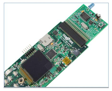
The idea is to make a universal remote controller with keypad and a small display. Command to learn and fire IR codes is not much different from that in part one of this manual when COM Port of a PC is used, except that UART of the MCU now interfaces directly to C0168 IC of ULRC.
